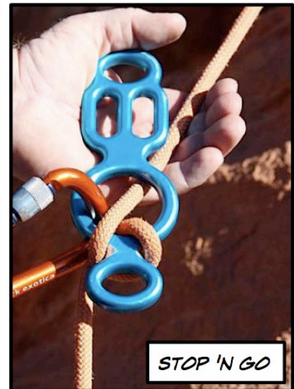
RIGGING WITHOUT OPENING THE CARABINER.
